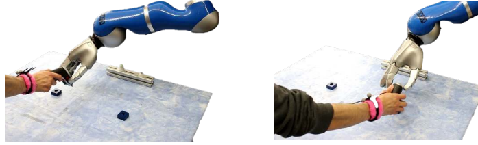
Fig. 6 Handover and return of a screwdriver at different positions, obtained by conditioning the Interaction ProMP on the positions of the wrist marker.
